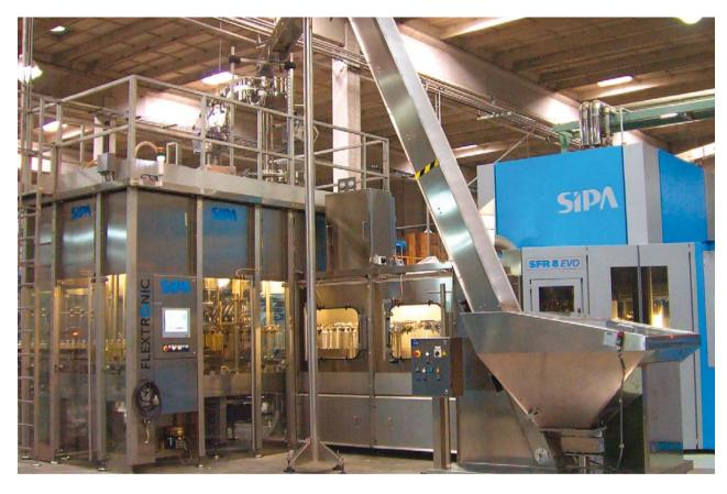
The Flextronic W is highly suited to lightweight bottles, as it handles them only by the neck. It also comes with the option of pressurizing the bottles with nitrogen in order to prevent the oil inside from oxidizing and losing its flavor. "Aceitera Martinez was very happy with the first line we installed, so it quickly chose the
