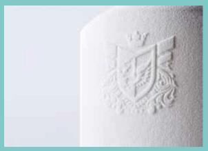
Enter additive manufacturing, better known these days as 3D printing. This is the ideal way to create your product prototype without having to cut any metal for your mold. Little more is needed than the digital (STL) file of the design, the 3D printer, and the printing material. Once set up, the actual process of creating your prototype takes just a few hours.
