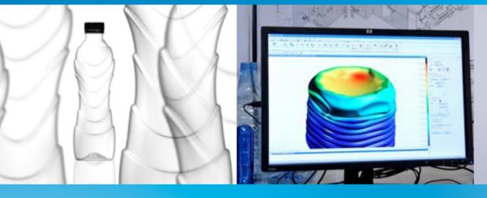
internal pressure resistance, and crushability. Different geometries can be compared, as well as different weights of the same geometry.
