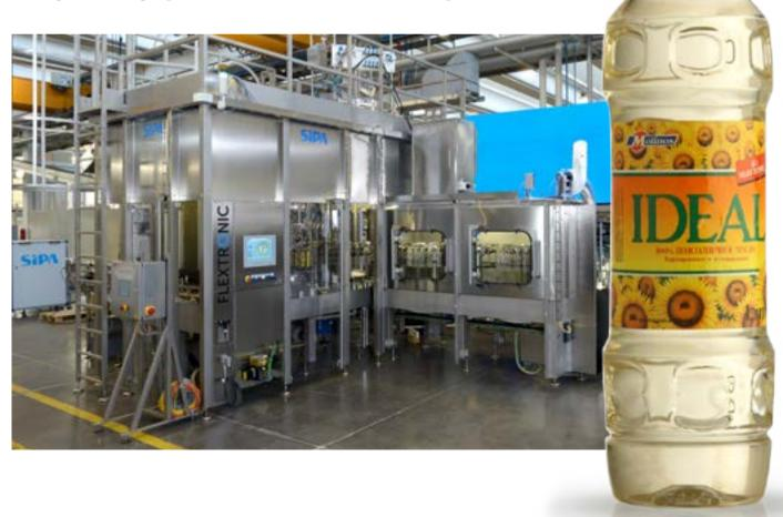
Thanks to new designs in the clamp unit and in the cams that have reduced moments of inertia, the SFR EVO3 has a maximum output rate of 2250 bottles per hour per cavity, which makes it highly competitive. The SFR EVO3 can be equip-
