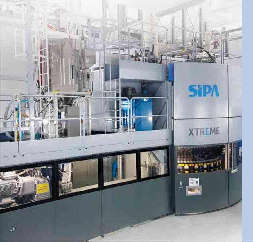
that used in conventional injection molding. The low-pressure production of preforms enables a weight reduction in every preform compared to the lightest injection molded preforms on the market today, creating important savings in production costs and, most importantly, in the amount of PET used thus reducing the environmental burden such as CO<sub>2</sub> emissions.
