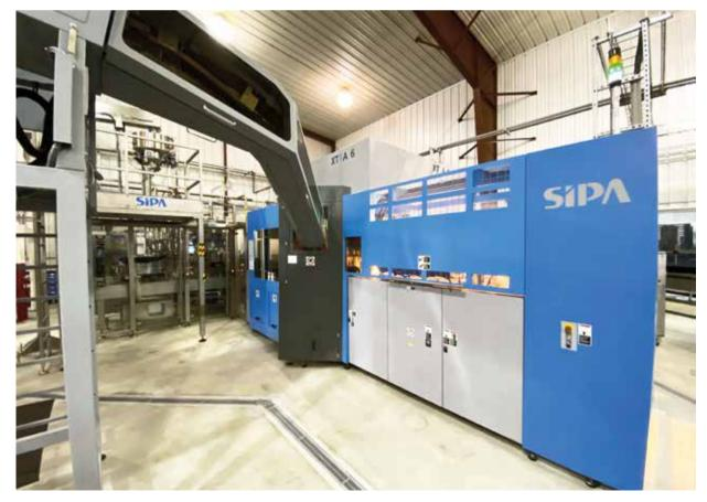
The Sincro Bloc system features very fast product changeover without the need for special tools. The line is equipped with an ECHO system for remote control and monitoring, enabling digital management.
