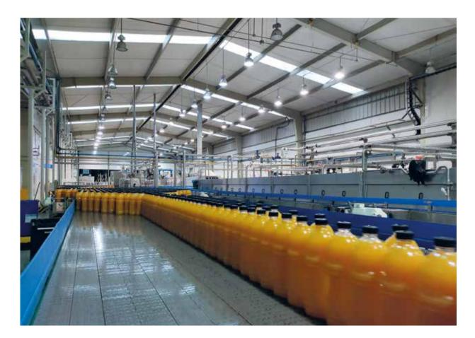
The Flextronic SE filling monobloc, equipped with "no contact", double speed shutter filling valves made in AISI 316L low-carbon stainless steel, is designed for hot-fill applications in ultraclean configurations.
