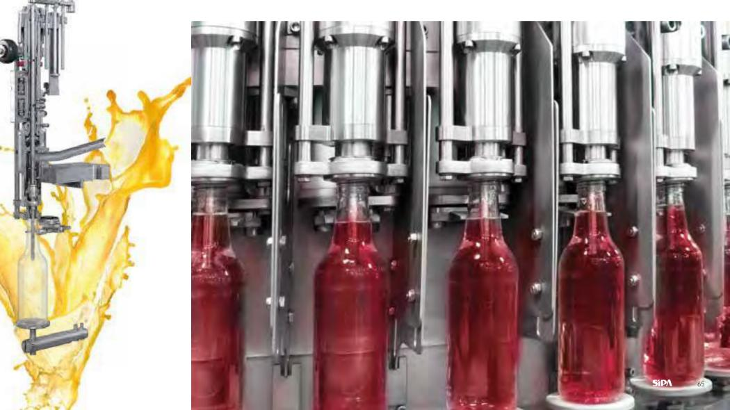
requirements. The SIPA entry level is ISO class 7, but this can be increased up to ISO class 5 if the customer requires it. Features that can be added include overpressure sterile air cabins with contamination control equipped with HEPA filters, and protection of the filling area with a mini-enclosure (isolator technology) for sensitive product handling.
