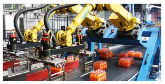
range of solutions for different container handling in plastic crates, American-type cartons and wraparound, designed to meet different levels of speed and to cover all production needs, from the simplest to the most complex packaging configurations handled with robotic solutions.
