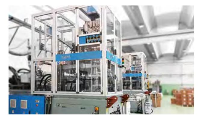
Ho.Bag has acquired two ECS SP 25 singlestage injection-stretch-blow molding systems, including numerous molds made by SIPA. Ho.Bag is using these machines to supply customers with a notable range of container sizes, shapes and colors, in small and very small lots – down to as low as 10,000 bottles per order.
