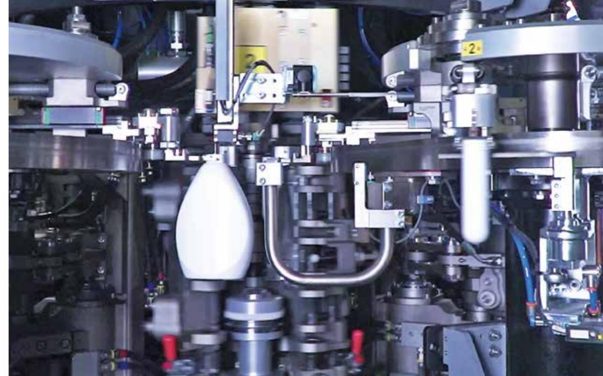
Each position in an XTRA PH oven has its own specific high-performance ventilation, with one fan for incoming filtered fresh air and four fans for hot air extraction, each one adjustable by a dedicated inverter. Meanwhile internal air cooling is done via special bored stretching rods with patterns of holes created according to the design of the bottle.
