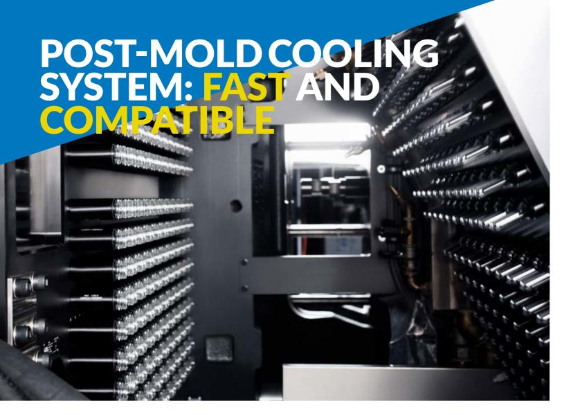
XFORM GEN4 features a post-mold cooling system which delivers unprecedented cooling efficiency and unique flexibility. The EOAT features up to 4 cooling stages for 30mm-neck preforms; legacy EOAT can also be installed on the GEN4 PMC systems.
