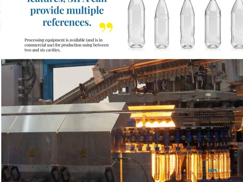
Diverse blow molding systems are in use for RefPET bottle production. For high output – up to approaching 8000 bph – of bottles around 2L in volume, there are the XTRA 6 and 8 rotary systems. Linear SFL systems – Performance 6, Dynamic 4 and Dynamic 3H, as well as Flex 2 types, with their best-in-class performance cater for lower outputs and larger bottle volumes.
