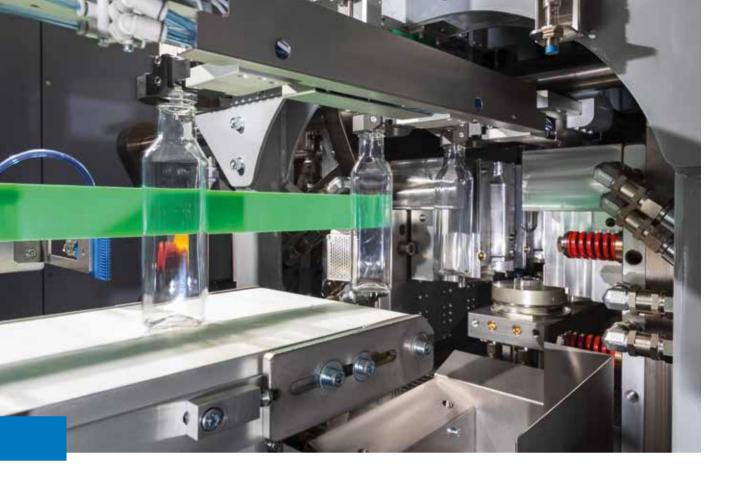
SIPA has introduced the SFL Flex machine, expanding its SFL range of linear stretchblow molding machines to cater to the production of small batches. The SFL Flex is available in two versions, one with two cavities and the other with just one. These machines are designed for lower output segments, producing between 1000 to 4000 bottles per hour.
